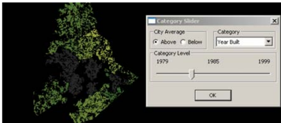
Fig. 5: The category slider locates buildings that fit a specific criterion. In this example, only buildings in Charlotte that are built after 1985 are shown.
